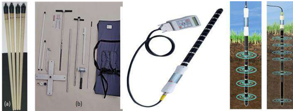
Fig. 2: Soil moisture profile probe installed at drought phenotyping locations.
